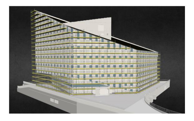
Scaffolding project for future construction of a building in Norway designed with PON CAD 3D software by RAMIRENT using Multidirectional Scaffolding system.
