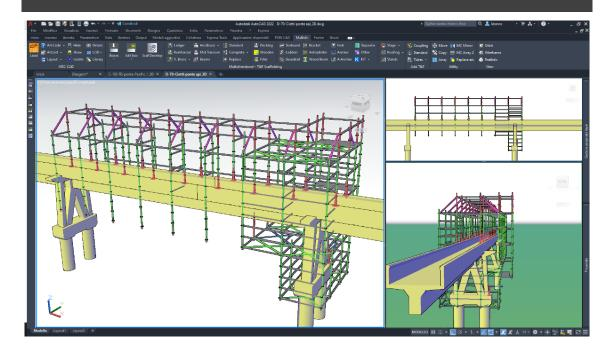
Suspended scaffolding designed by CIOTTI PONTEGGI with generic multidirectional library supplied in the standard package of PON CAD software.
